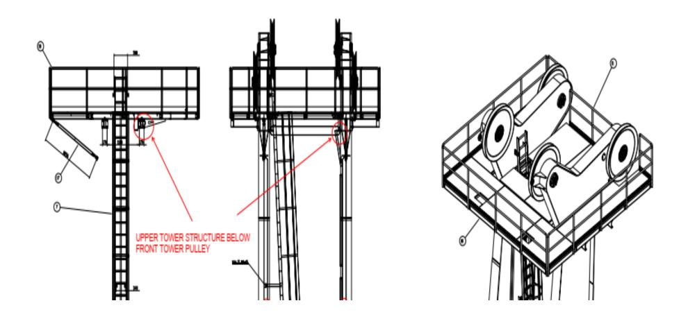
N. B.: The above marked areas (four locations) beneath the Tower Pulley Structure are to be checked/inspected for cracks by carrying out Non-Destructive Testing and to be rectified by welding, in case of any cracks.
