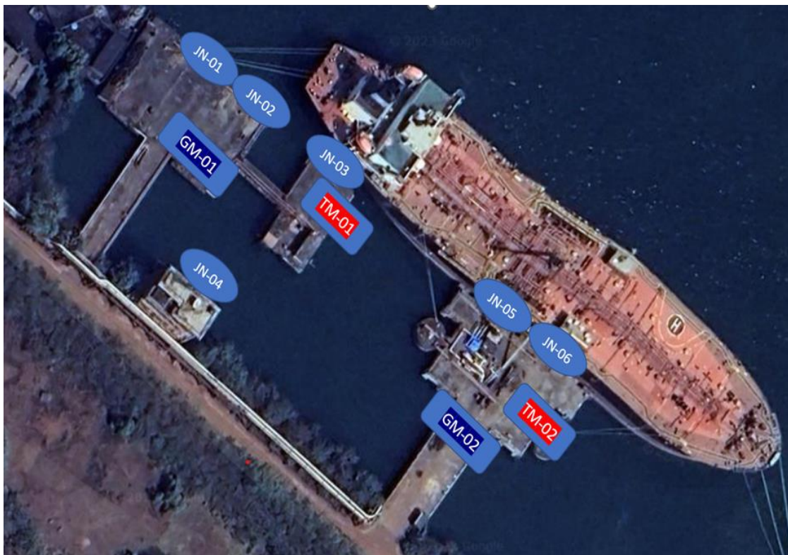
Figure-1: Jumbo Nozzles, Tower Monitors and Ground Monitors locations
