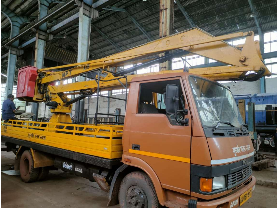
Ladder Mounted Crane
